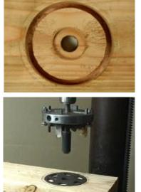
4. When complete, the grooves created by the dapping tool should be at the proper depth so that the face of the **shear plate** sits flush with the surface of the wood. Adjust the depth accordingly if the shear plate sits too high or too low in the grooves.
