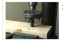
**3.** Insert the **dapping tool** into the handheld drill or drill press. Use the **pilot bit** to align the **cutter head** with the pre-drilled bolt hole. Small cap screws on the face of the dapping tool can be adjusted to change the depth of the grooves.
