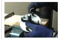
**1.** Assemble the 3/4" **pilot bit** into the **cutter head** and tighten it with an **Allen wrench**. Set the dapping tool aside.
