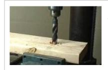
2. Drill a 13/16" bolt hole in the wood. A drill press is used in the video, but a heavy duty, 3/4" or larger handheld portable drill will work.
